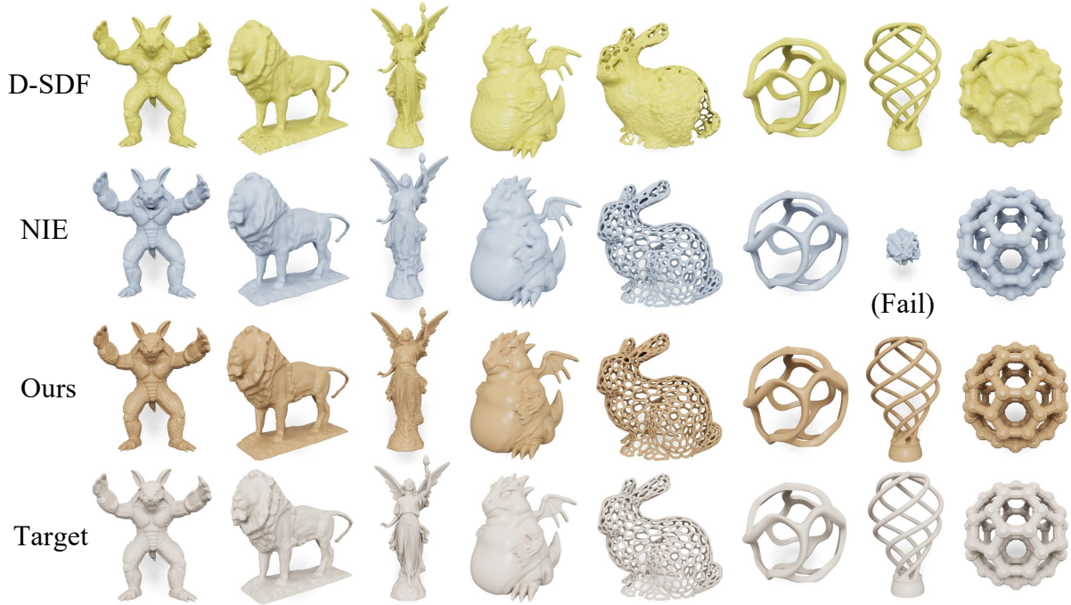
Fig. 17. Inverse rendering experiments compare our method with D-SDF and NIE across 8 different shapes. The first four columns display geometrically complex shapes, while the last four show topologically complex shapes. This demonstrates that our method surpasses the compared approaches in detail preservation and topology correctness.
